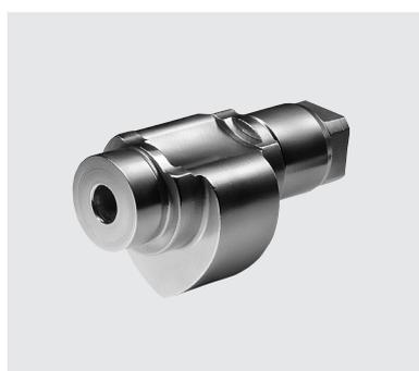
The heart-shaped cam and linear drive mechanism of the TS 97 ensure that the resistance encountered decreases almost instantly with the door opening action – so even children, the elderly and people with disabilities have no problem in passing through. User-friendly and reliable closing is also ensured by the delayed increase in the actuating torque at the 'latching' end of the sweep.
